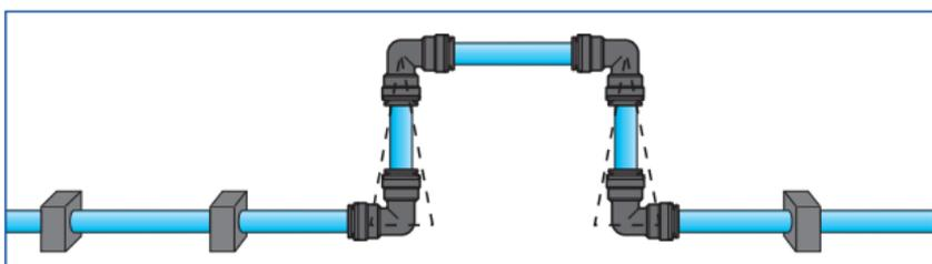
On long pipe runs, it is advisable to install an expansion bend, as shown in the diagram.
