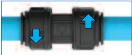
**To disconnect**, turn the screw cap 1/4 turn, push in the collet and remove the pipe. The fitting and pipe can be reused.
