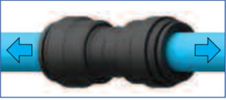
**To disconnect,** ensure the system is depressurised. Push the collet towards the fitting and remove the pipe. The fitting can be reused.
