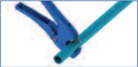
**DO NOT** use a hacksaw. To avoid damage to the 'O' ring remove burrs and sharp edges.
