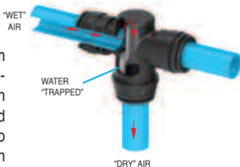
The ingenious inside arrangement of the fitting allows air to flow, with minimum head loss, from the main to take-off point without allowing water to follow. The moisture is retained in the line to be drawn off at some suitable location.
